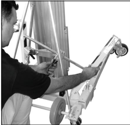
To replace the leg in the stowed position, pinch the locking mechanism release and fold the leg up.
