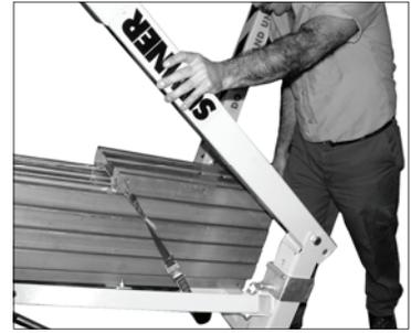
While holding the leg in the 90 degree position, slide the Leg Lock back towards the leg until the spring load-ed plunger pin engages into position.
