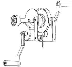
10. Wind the slack cable tightly and evenly across the load drum.
