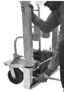
Insert extension legs into operating position by raising plunger pin and sliding leg into socket until plunger pin is fully engaged. Repeat for second leg.
