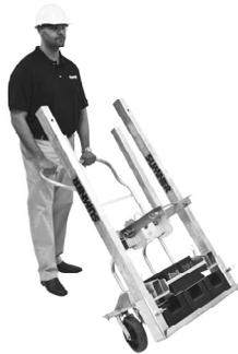
The lift comes equipped with a steering handle. The handle makes moving the lift around the jobsite easier.
