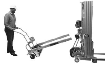
Pull up on the plunger ring and slide Lock Block back over extension leg until plunger locks into position.
