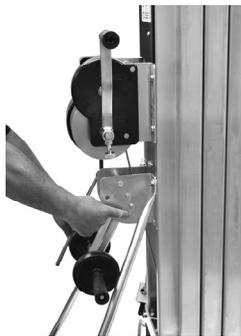
To extend the handle, press down on the spring loaded pin and rotate the handle up. The spring loaded pin will lock the handle into the extended position.
