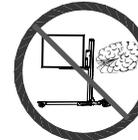
Never operate in gusty winds. Lifting loads during high winds can result in the lift tipping over and the possibility of operator injury.
