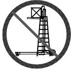
Do not climb on mast or put a side load on mast. Do not use unit to support ladders for climbing or hoisting.
