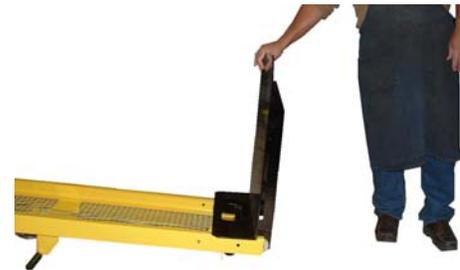
**Step 1.** To assemble your lift, first lay down all three pieces on the floor or table for easy viewing of the components. Lay the mast assembly on its back (winch side). Slide the tray into the mast from the bottom.
