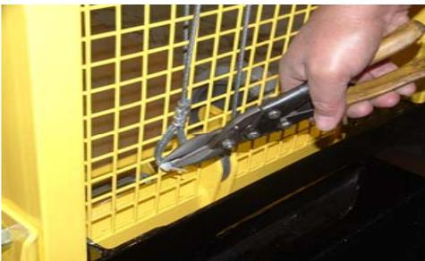
**Step 7.** Cut plastic tie holding lifting cable.
