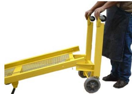
**Step 3.** Next, insert base into the mast as shown. Secure the tray to prevent it from sliding down during this operation.
