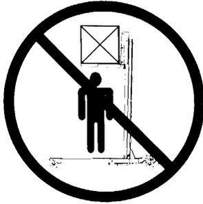
Do not misuse the unit. Perform only the functions for which the unit is designed. Never attempt to operate the equipment at more than the recommended capacity.
