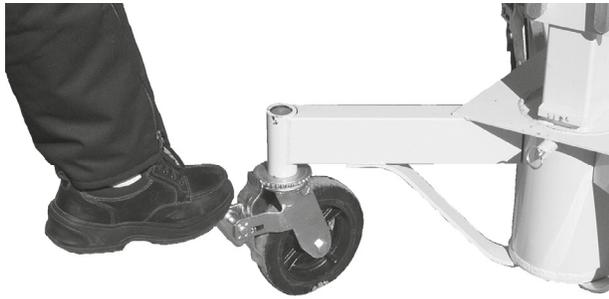
1. Set brake by pressing down on brake lever as shown.
