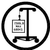
Test load balance before lifting. Do not exceed rated load capacity. Never use two Roust-A-Bouts to lift a load which exceeds the capacity of a single lift.
