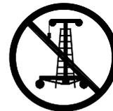
Do not climb on Roust-A-Bout or put side load on mast.
