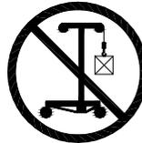
Never lift a load over the short legs unless a counter weight equal to the load is applied to the long legs.
