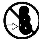
Never lower load using free fall lever. Keep lever engaged at all times under loaded conditions.
