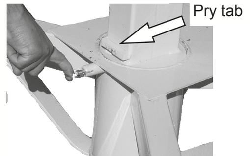
2. Place crowbar under pry tab and raise mast from base until the locating ring rests on top of the base.
