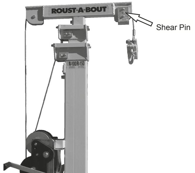
**Note:** All R-Series Roust-A-Bouts contain a safety device known as a Shear Pin. This pin is located on the front sheave of the "Tee Head". The purpose of the pin is to protect the lift in the event of an overload. A spare Shear Pin is located underneath the Winch Assembly.
