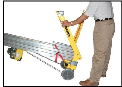
While holding the leg in the 90 degree position, slide the Leg Lock back towards the leg until the spring loaded plunger pin engages into position.
