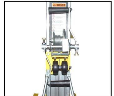
The winch handles have been placed in the stored position.
